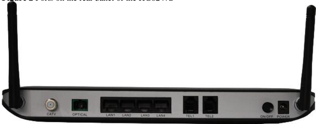
Figure 2 Ports on the rear panel of the HG8247a
