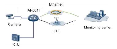
Huawei AR631I-LTE4EA can be deployed to provide 4G/3G wireless backhaul for cameras in areas where conventional wired coverage is difficult. It can also offer 4G backhaul in industrial manufacturing scenarios. Due to highly reliable industrial design, AR631I-LTE4EA ensures secure and reliable network communication in challenging environments with extreme temperature, humidity, and electromagnetic interference.
